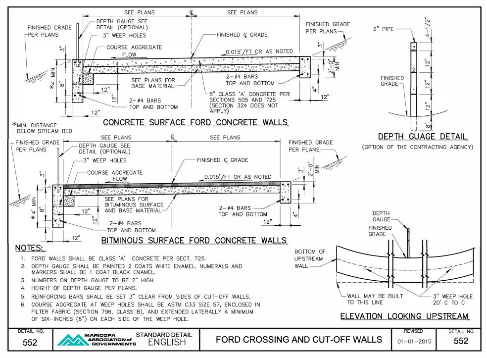
Construct (200' x 25') Concrete surface ford (low water crossing) per Mag Standard Detail 552. 8" Concrete on 4" Aggregate Base Course. Including depth gauge. Crossing profile grades shall match existing wash profiles. Extents of crossing will be marked in the field by the Town prior to construction. Campbell Road and Carlisle Wash.
